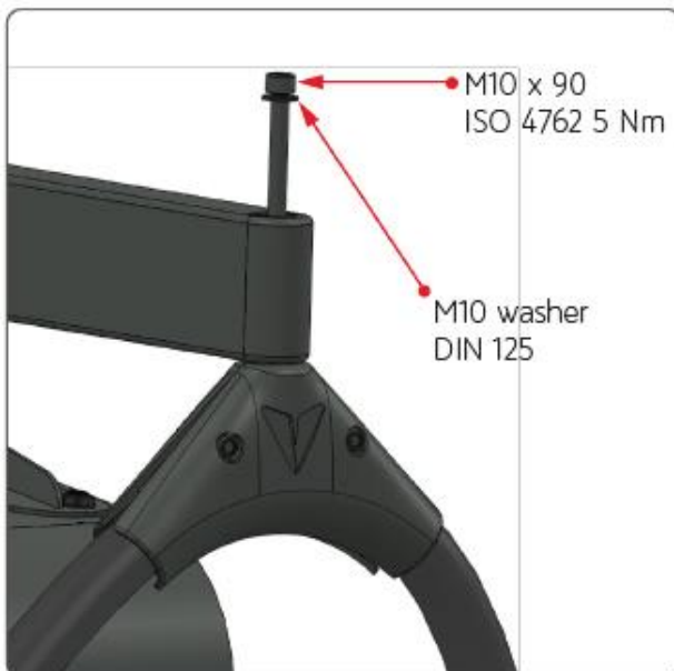
Figure 12: Used fixings
